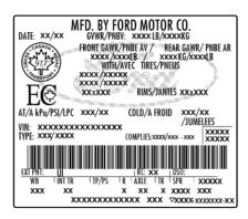
**WARNING:** Exceeding the Safety Compliance Certification Label vehicle weight rating limits could result in substandard vehicle handling or performance, engine, transmission and/or structural damage, serious damage to the vehicle, loss of control and personal injury.
